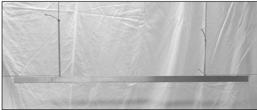
Figure 3: Aluminum beam and support system.
