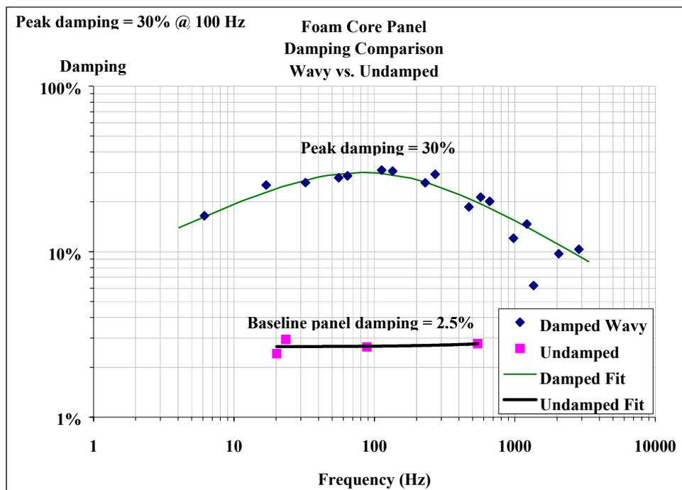
Figure 12: Test data showing damping measurements of wavy damped panel vs. equivalent undamped panel.
