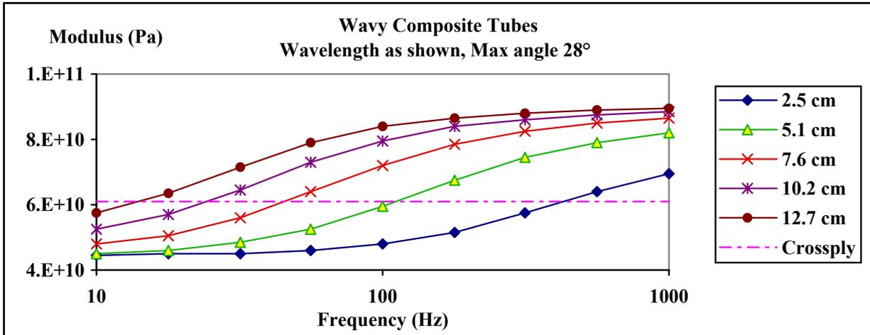
Figure 3: Equivalent axial modulus for carbon fiber wavy composite – viscoelastic tube.
