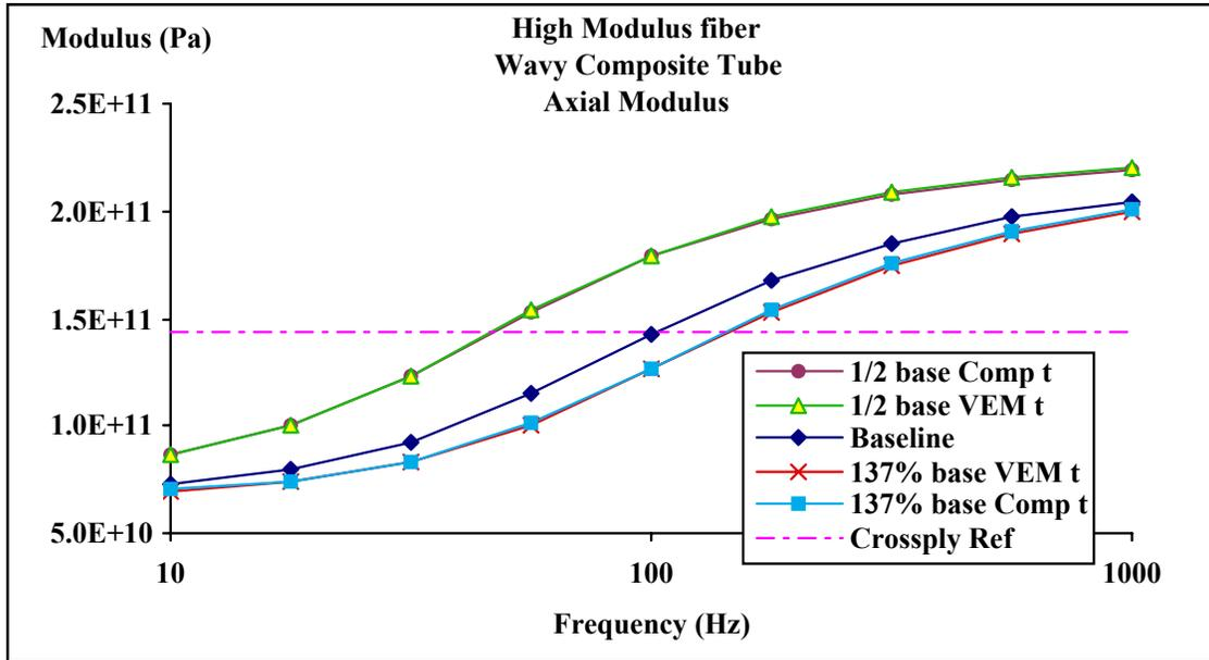
Figure 8: Effects of changing thickness of composite or viscoelastic layers on stiffness.
