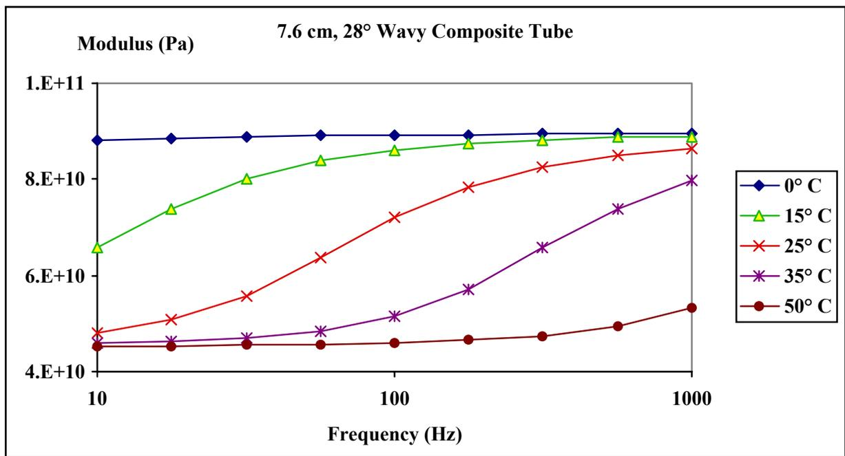
Figure 6: Frequency shift of the stiffness curve due to temperature.
