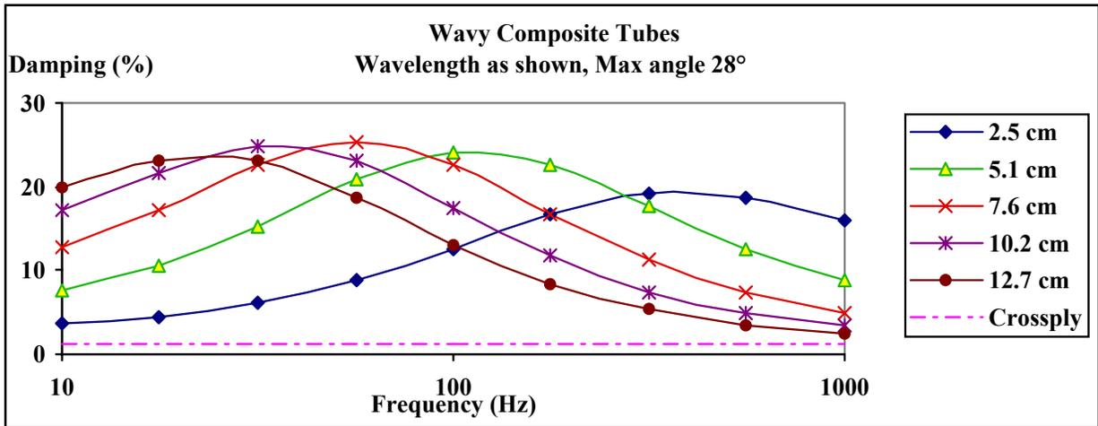
Figure 4: Damping (%) performance for carbon fiber wavy composite – viscoelastic tube.
