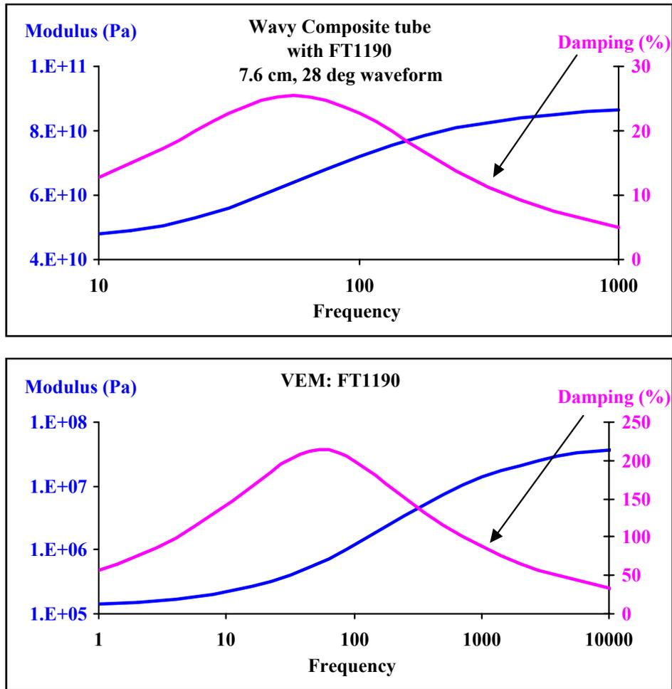
Figure 2: Modulus and damping of wavy composite tube made with FT1190 VEM (upper chart) compared with FT1190 series viscoelastic properties at 25° C (lower chart).
