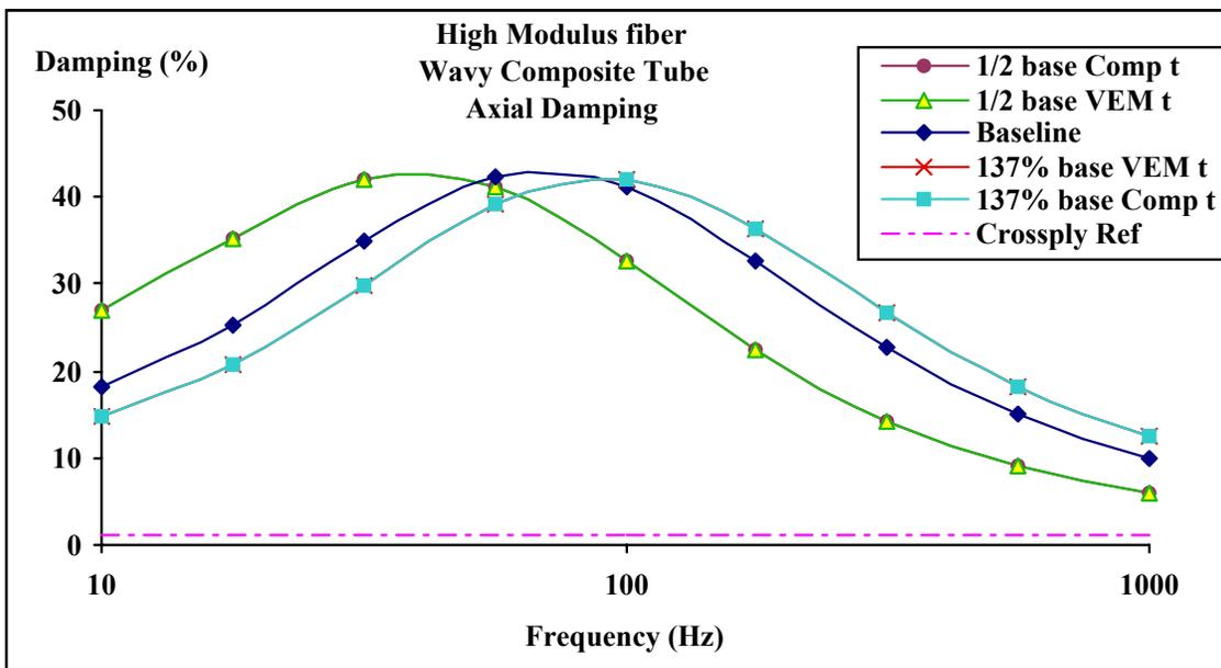
Figure 9: Effects of changing thickness of composite or viscoelastic layers on damping.
