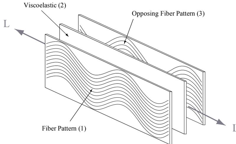
Figure 1: Basic damped wavy composite concept
