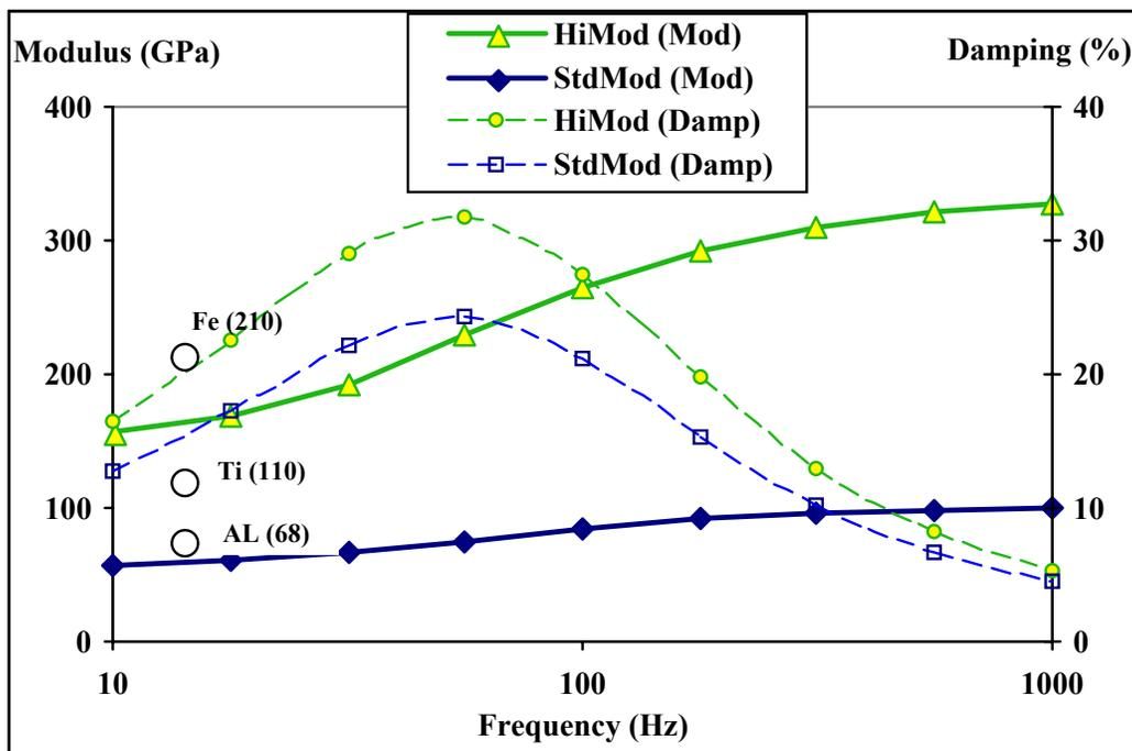
Figure 11: Comparison between high modulus fiber (K13710) and standard carbon fibers.
