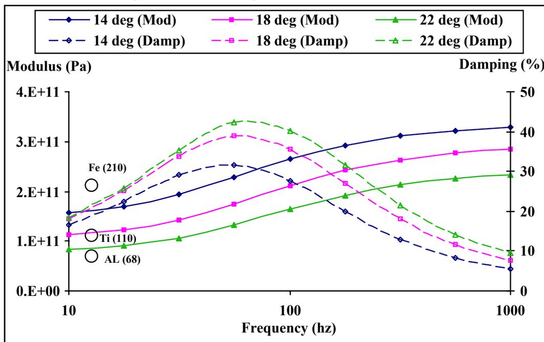
Figure 10: High modulus fiber based wavy composite tube axial modulus and damping performance at different maximum angles, wavelength 7.6 cm
