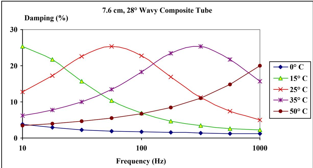
Figure 7: Shift in damping peak due to changes in temperature
