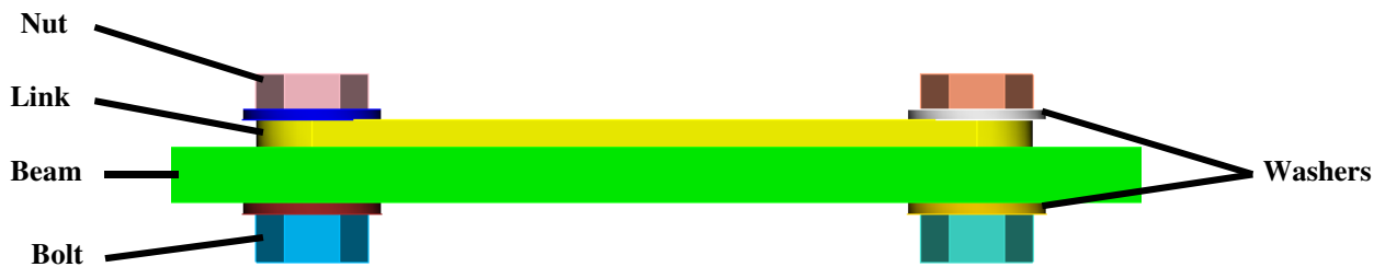
Fig. 12 Schematic of the link and beam connection that was used in the experimental setup.
