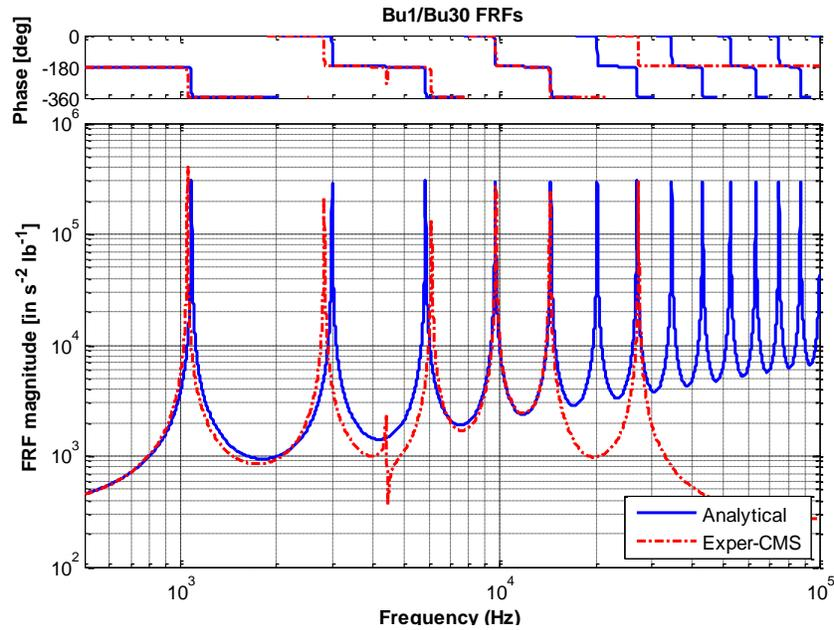
Figure 8: Frequency response function of beam in bending direction after removing the transmission simulator. The blue line shows the analytical FRF computed from the FEA model of the beam alone, while the red line shows that of the substructure model after eliminating the negative eigenvalues using the ad-hoc approach.
