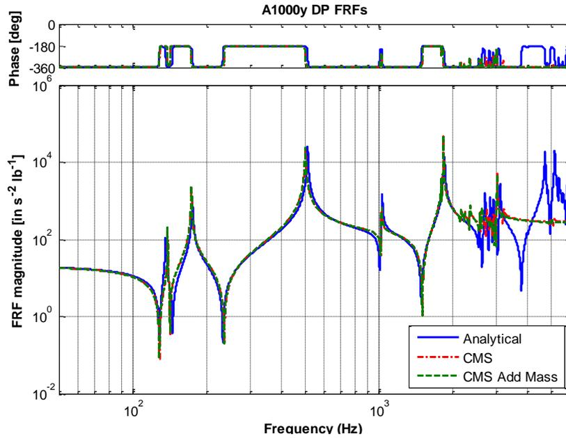
Figure 5: Frequency response function of the assembled system at the drive point labeled 1000y (axial direction). The blue line shows the analytical FRF of a finite element truth model. The other lines show the FRFs estimated by modal substructuring, the red is the baseline model that has negative mass while the green is from a model that was corrected using the added mass algorithm in Sec. 3.1.2.
