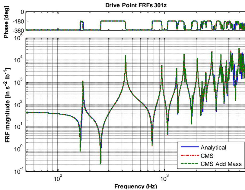
Figure 6: Frequency response function of the assembled system at the drive point labeled 301z (radial direction). (See description for Fig. 5)
