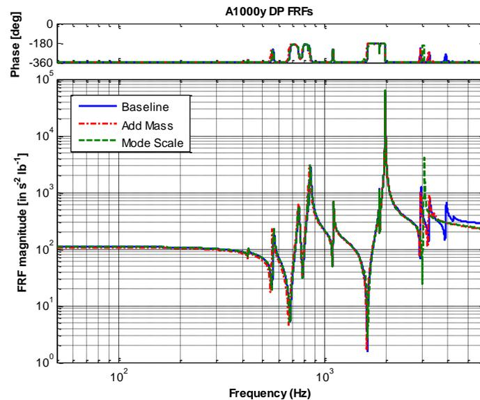
Figure 7: Blue curve provides the analytical axial C-A plate/beam FRF, red is the added mass method and green is the mode scale factor method for generating positive definite mass matrix after subtraction
