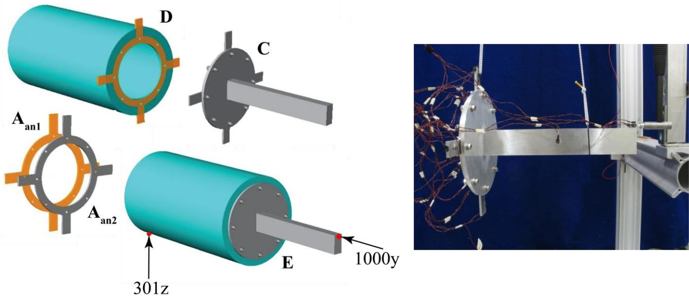
Figure 4: Schematic of Cylinder-Plate System and photograph of the hardware that was tested to obtain an experimental model for substructure C. Labels are shown indicating the names of the substructures, as well as two drive points where FRFs were later reconstructed.
