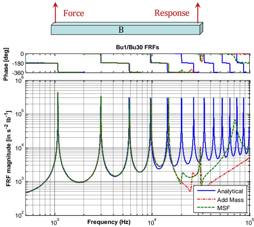
Figure 2: Frequency response function of beam in bending direction after removing the transmission simulator. The blue line shows the analytical FRF computed from the FEA model of the beam alone, while the red and green lines show those of the substructure model estimated after removing the transmission simulator and after adjusting the mass matrix using the Added Mass and Modal Scale Factor approaches.
