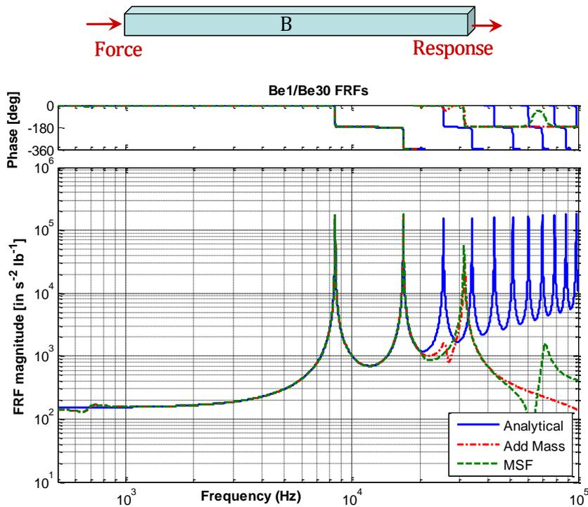
Figure 3: Frequency response function in the axial direction. (See description for Fig. 2)
