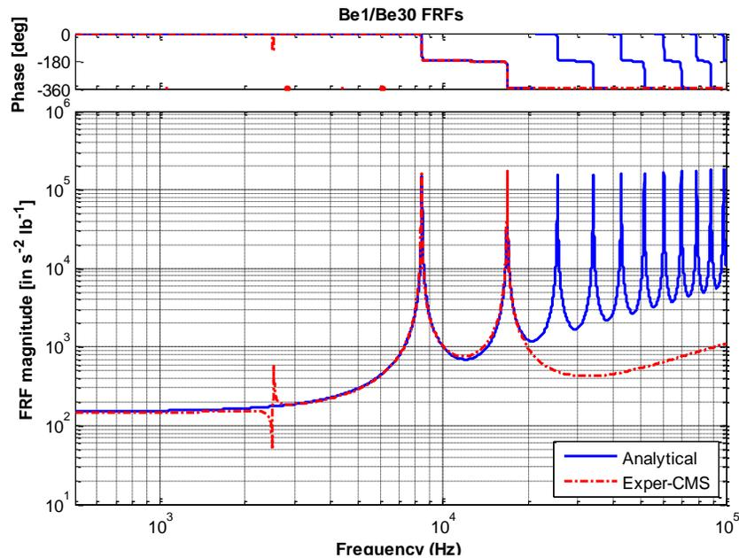
Figure 9: Frequency response function in the axial direction. (See description for Fig. 8)
