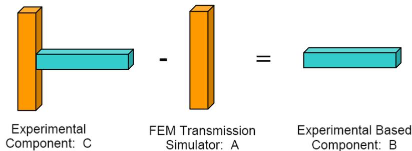
**Figure 1:** T-Beam System. The substructure of interest is the (blue) horizontal beam. It is tested while connected to the (orange) vertical beam, or transmission simulator. The proposed procedures will be used to obtain a positive definite mass matrix after removing the transmission simulator.
