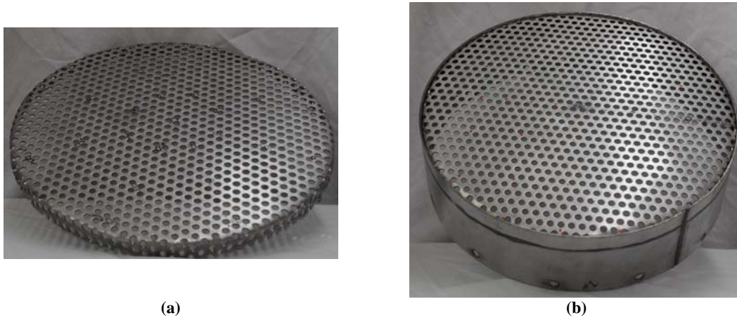
Figure 2: Experimental setup of the perforated plates. a) Perforated plate before welding into test configuration, b) Perforated plate welded into the supporting cylinder.
