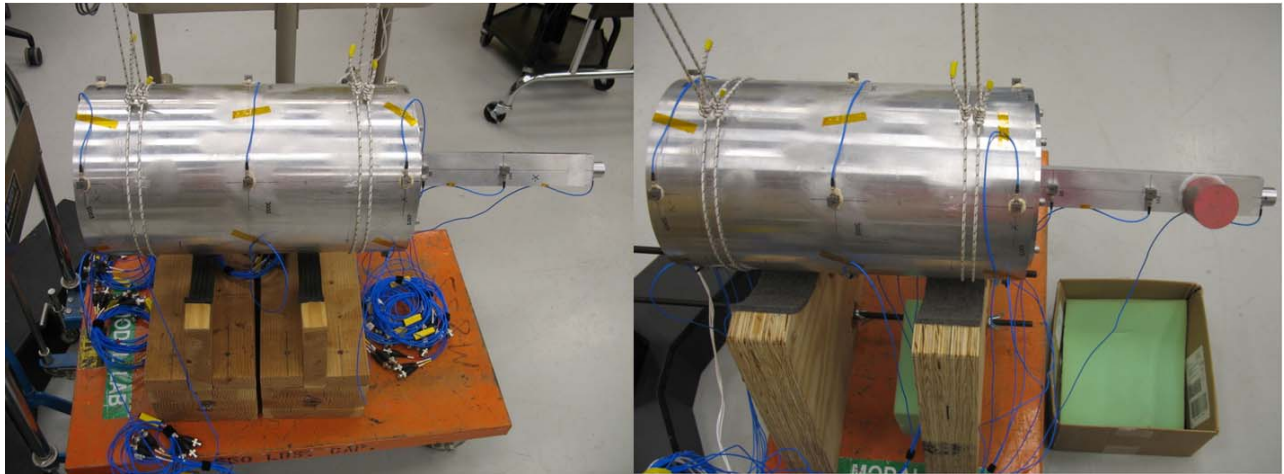
Figure 7: Experimental setup for system C (left) validation test on system E with added mass (right)
