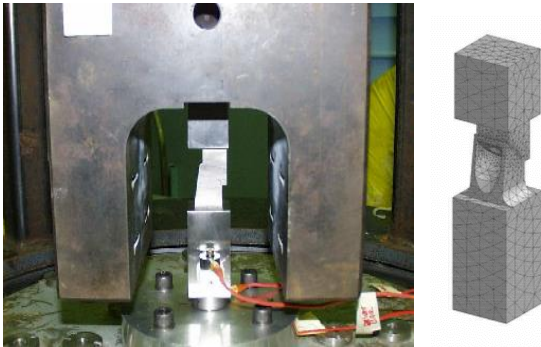
Fig. 1: Photograph of experimental setup used to measure dissipation in a lap joint. A finite element representation of the joint itself is shown on the right.
