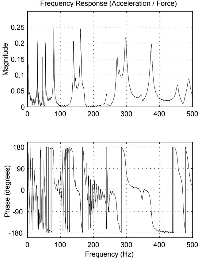
Figure 2: Typical Frequency Response for impulse tests of square plate.
