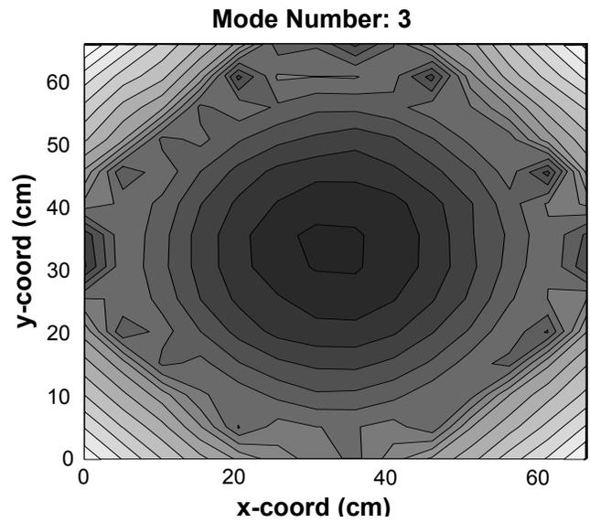
Figure9: Contour plot of third mode-STAR.
