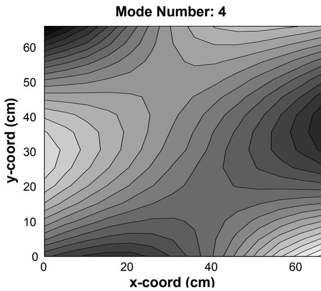
Figure10: Contour plot of fourth mode-LLS-SDOF.
