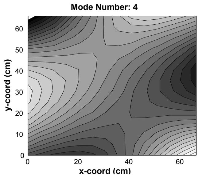
Figure11: Contour plot of fourth mode-STAR.
