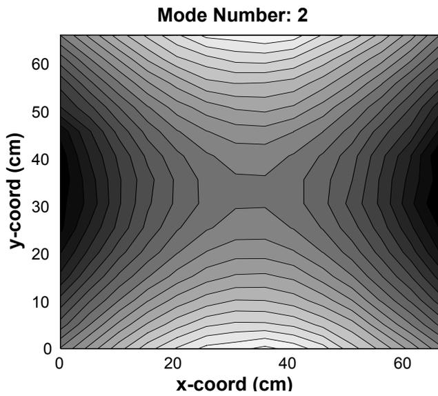
Figure 6: Contour plot of second mode-LLS-SDOF.
