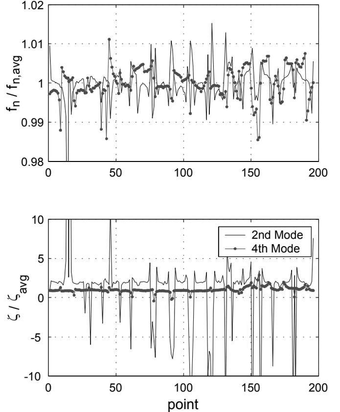
Figure 3: Point to point variation in natural frequency and damping ratio for AMI-SDOF algorithm.
