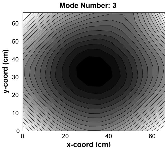
Figure8: Contour plot of third mode-LLS-SDOF.
