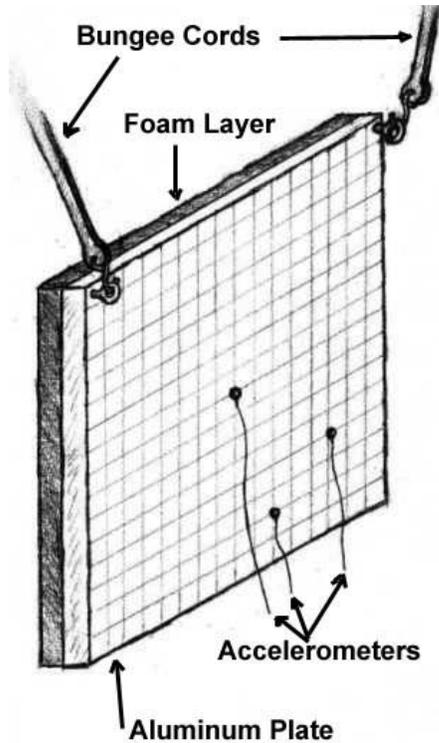
Figure 1: The experimental test specimen - a free square, aluminium plate with unconstrained foam layer.
