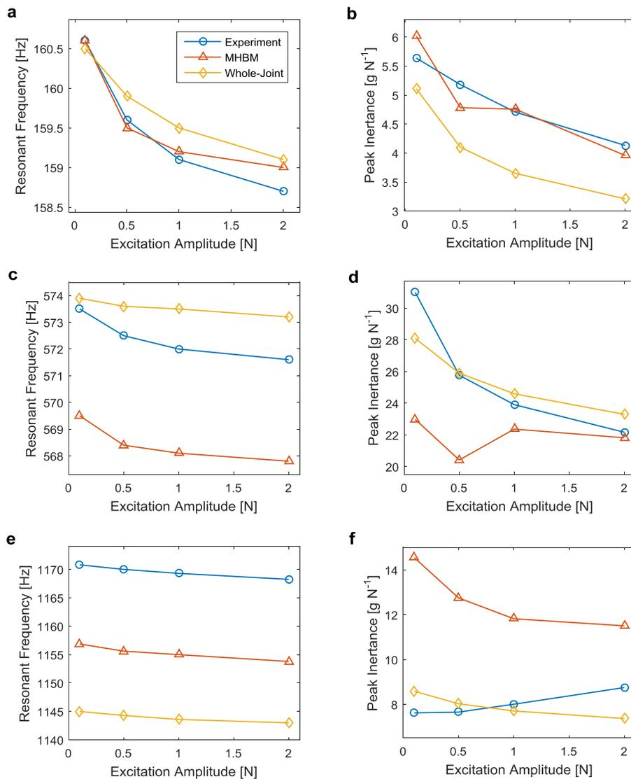
**Fig. 1** Comparison between experiment and the modeling approaches of (a,c,e) the resonant frequency and (b,d,f) peak inertances in the (a,b) first, (c,d) second, and (e,f) third bending modes of the Brake-Reuss beam.
